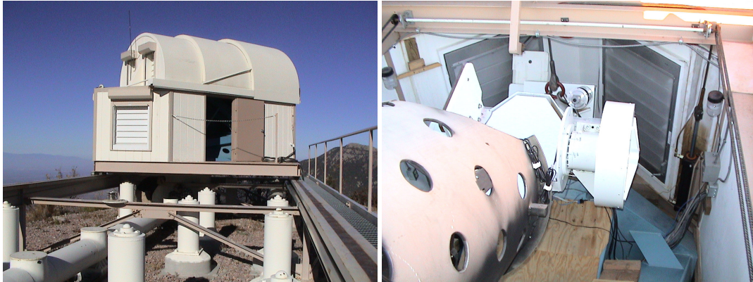
Figure 3.2: Left: The dome of telescope A in closed position. Right: The siderostat which feeds the CASSEGRAIN optics (the tube to the left).
